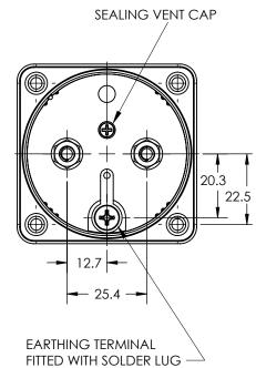
RECOMMENDED PANEL HOLE CUT-OUT: Ø 54.0 mm
